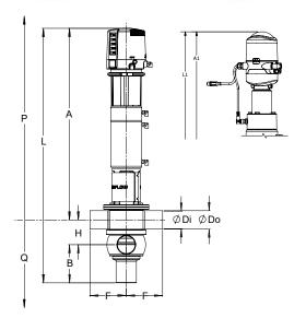
NOTE: Add the following approximate dimension to "F" for each clamp port connection: 0.5" for valve sizes 1.5" - 3.0", 0.62" for valve size 4".
